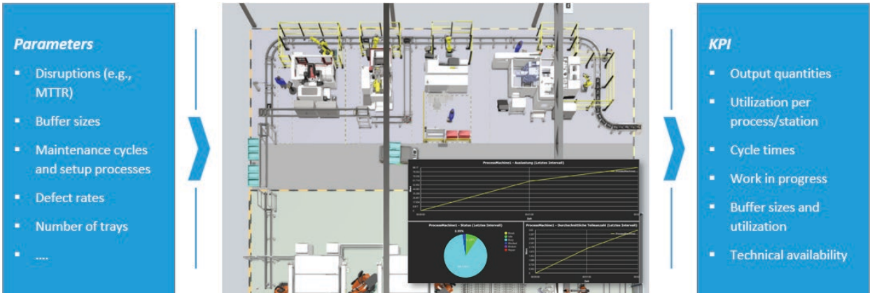
Figure 2: Parameters and KPIs for the material flow simulation
